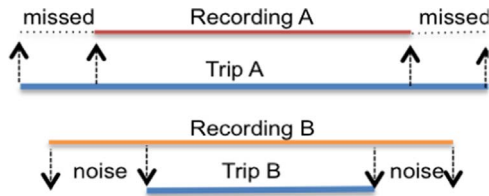
Fig. 4. (Top) Completeness of recordings measures the percentage of a trip being recorded and labeled. (Bottom) Precision of recordings measures the percentage of a recording that precisely reflects its label.
